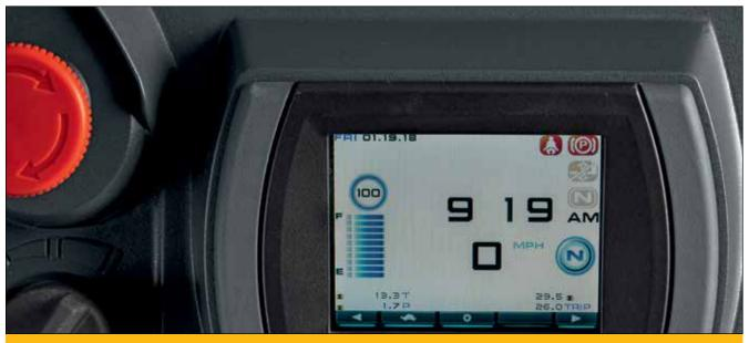
The display includes date, clock, speedometer, vehicle hour meter, warning icons and more.
